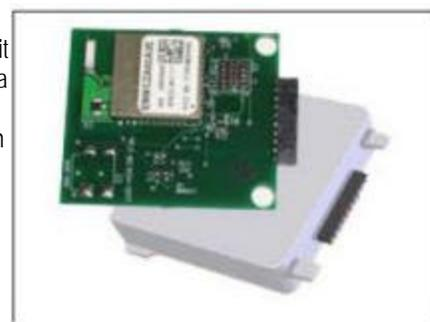
The user-replaceable U-SNAP module shown here measures only 1.5 inches (3.8 cm) square. The plastic enclosure protects the circuitry while providing convenient access from the exterior of the device. A HAN Device Portal designed to use plug-in U-SNAP modules offers the consumer greater flexibility while offering the utility a future-proof approach to the HAN.
