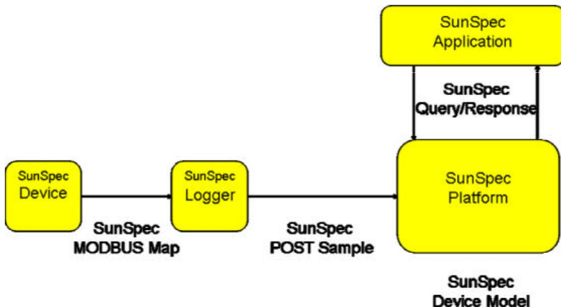
*The SunSpec Alliance Architecture, which includes both specifications and Reference Implementations, creates a Common Data Model for applications to communicate with multiple devices via existing networking protocols. Initially offered for inverters, meters and environmental sensors communicating via Modbus, the Common Data Model is extensible to other devices and network protocols.*
